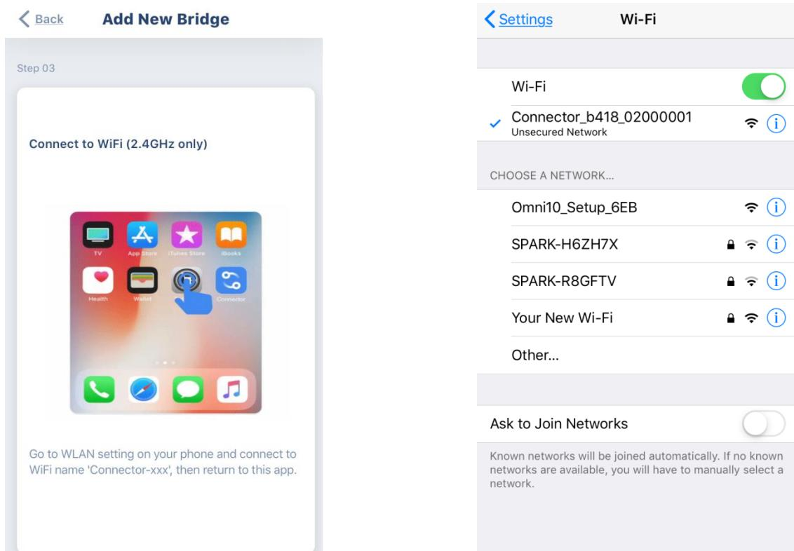
10. Return to the Connector+ mobile app and it should say "Connecting Bridge", which could take 1-2 minutes and a countdown to 0 will be displayed. At this time the light on the USB bridge will flash purple, green and finally blue
