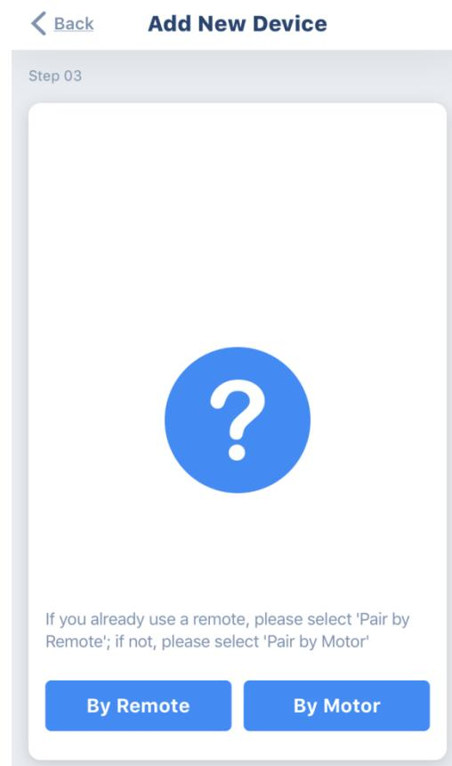
20. Follow the instructions on the screen. Locate and press P2 (on the back of the remote) twice, with a short space between the presses; the motor will jog up and down each time you press. Then press "Next". The blind is now pairing from the remote. There will be a 30 second countdown on screen
