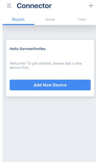
5. Select "Add New Device" and click on the image of the SmartLink USB bridge (top right image)
